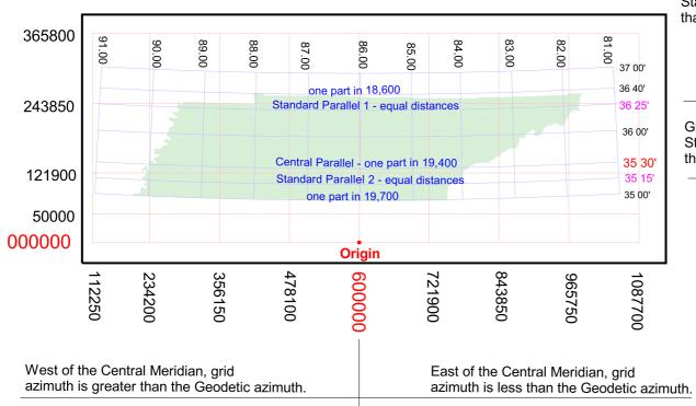
Grid distances outside the Standard Parallels are greater than the Geodetic distances.
